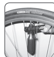
Figure 7. Inflating the tire with the cartridge in the upright position
