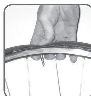
Figure 2. Squeeze the tire to extend the valve
