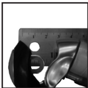
Figure 7- Minimum lever opening
